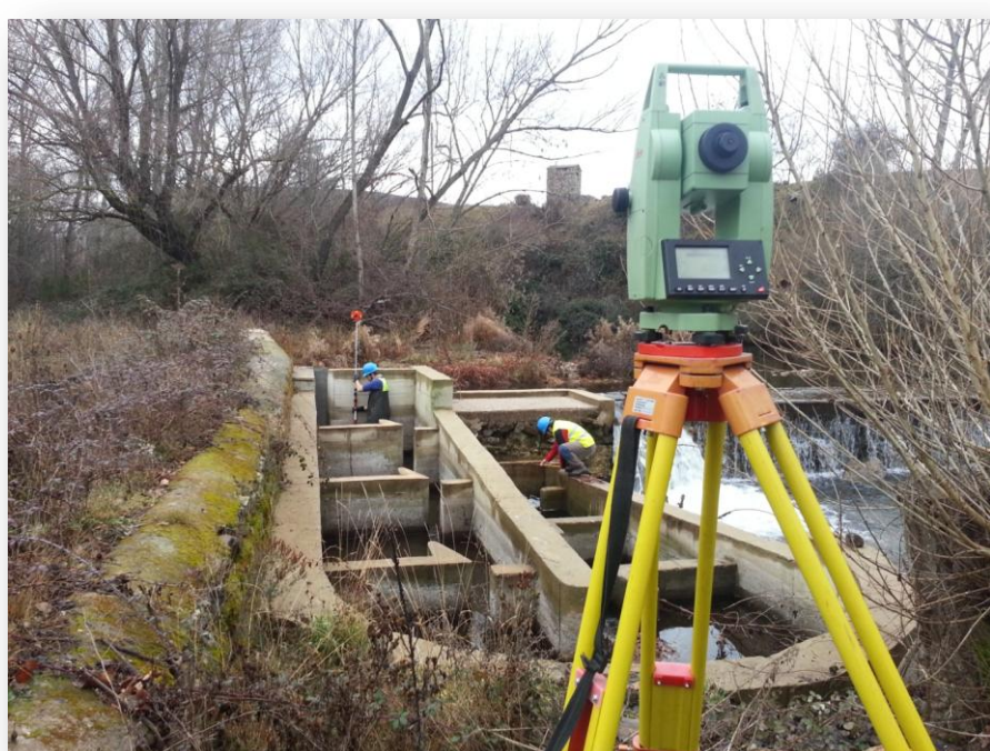
Figure 3. Topographic data collection is the first step to assess a fish pass.
